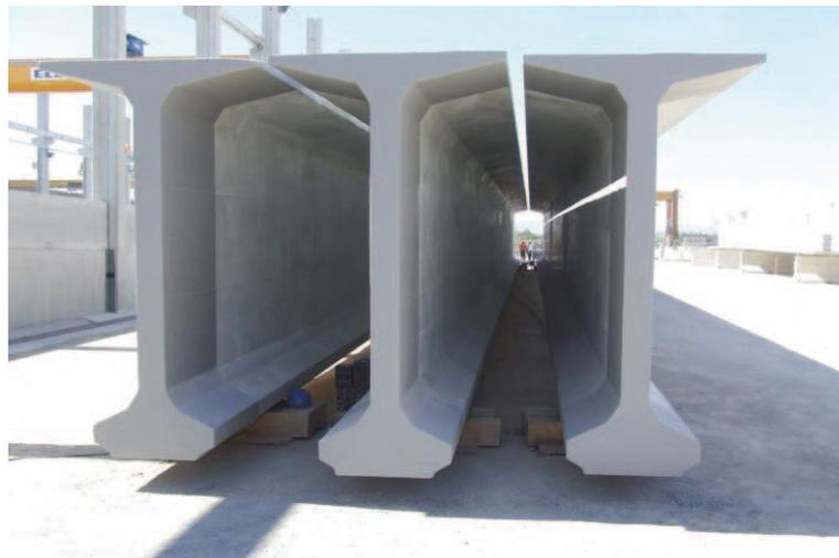
**Figure 2:** I section beam. One of the most common profiles to design and build the deck bridge
