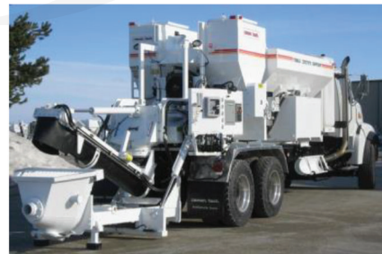
Fig. 4.6—Rotating drum and volumetric-measuring continuous-mixing (VMCM) units with pump. (Photos courtesy of: (a) Putzmeister; and (b) Cemen Tech.)
