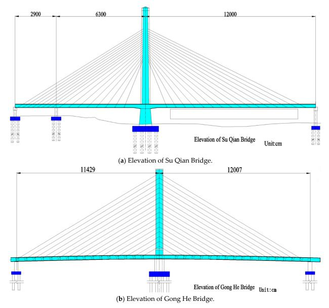
Figure 6. Schematic diagram of two bridges.
