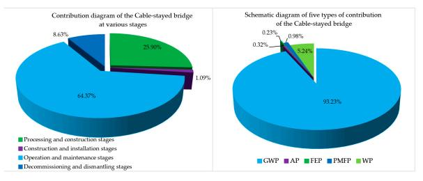
**Figure 8.** Schematic diagram of the environmental impact contribution of the four phases of the cablestayed bridge.
