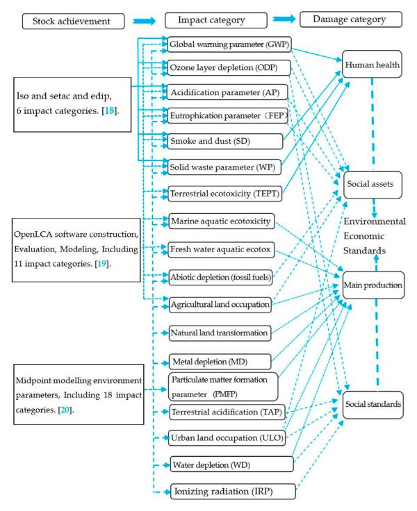
**Figure 2.** Schematic diagram of inventory and damage categories of construction materials' life cycle list. ISO: International Organization for Standardization, SETAC: International Society for Environmental Toxicology and Chemistry, EDIP: Danish Industrial Product Environmental Design Method.
