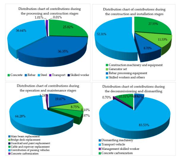
**Figure 7.** Schematic diagram of the environmental impact contribution of each stage of the cable-stayed bridge.
