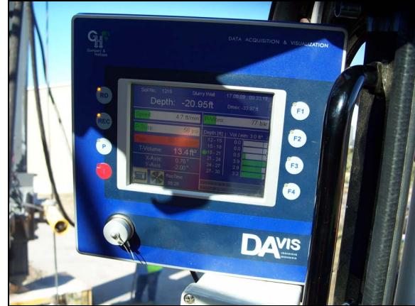
Photo 5 - Data acquisition system display mounted in cab of crane.
