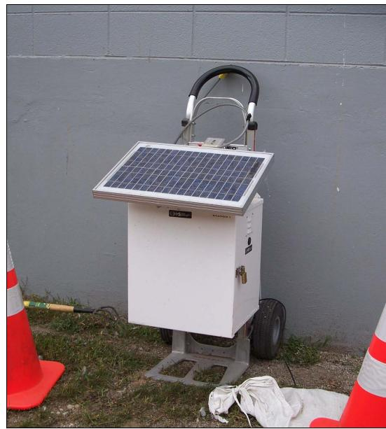
Photo 6 - Portable vibration monitors.
