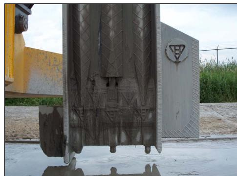
Photo 2 - Close-up of beam tip showing 10-inch fin and injection nozzles.
