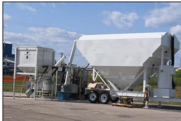
Photo 3 - Automated batch plant and reagent silos.
